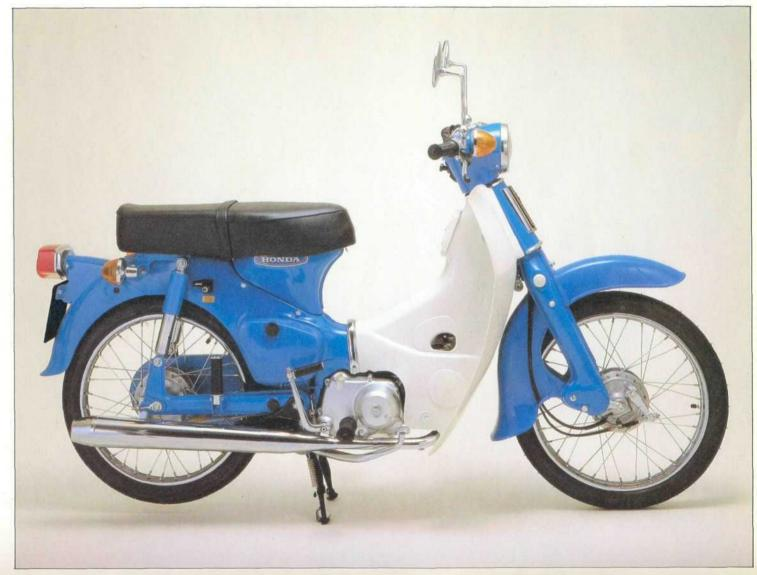
The C70 is the 72cc version of the step-through range, with an air cooled O.H.C. 4 stroke single cylinder engine, offering all the advantages of the C50 with a larger engine size.
